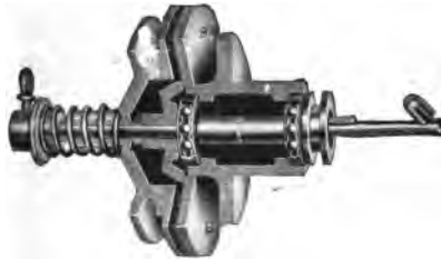
Showing the take-up mechanism of Powers machine
